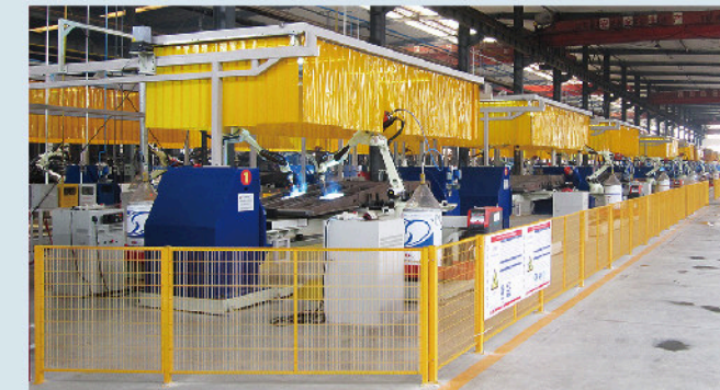
Fully automated welding workshop
