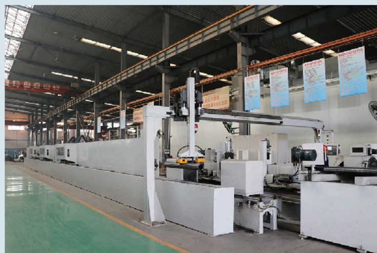
Automatic idler production line
